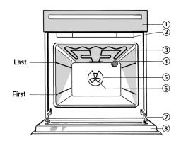
Note: The cooling fan switches on only when the oven has reached a certain temperature with the exception of the Grill Functions where it starts immediately.
