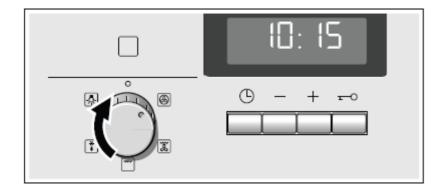
Set the temperature or grill using the temperature selector
