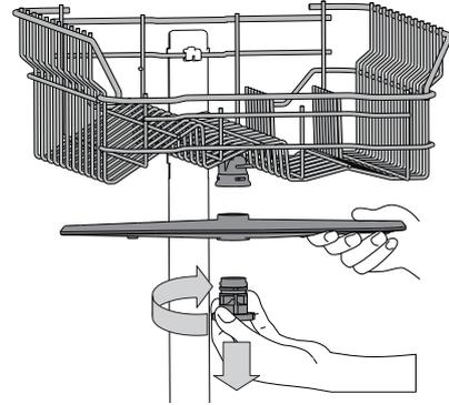
To remove the upper spray arm, turn the plastic locking ring in a clockwise direction. The upper spray arm should be replaced so that the side with the greater number of holes is facing upwards.
