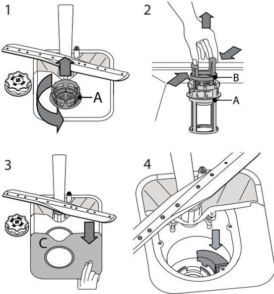
After cleaning the filters, re-place the filter assembly and fix it in position correctly; this is essential for maintaining the efficient operation of the dishwasher.
